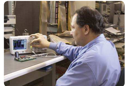
Figure 3. Standard go/no-go mask testing is just one of the reasons manufacturing and service test demand 1000 Series solutions.
